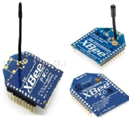
Figure 2.11: Wire Antenna Xbee Pro 60 mW Series 1(802.15.4)
